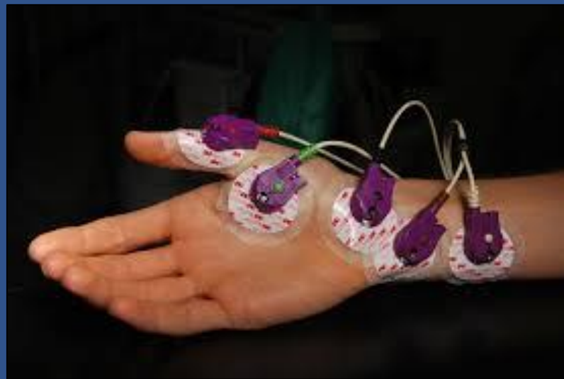
Fig 8.1: An example of electromyography (EMG) sensors placed on hand.
